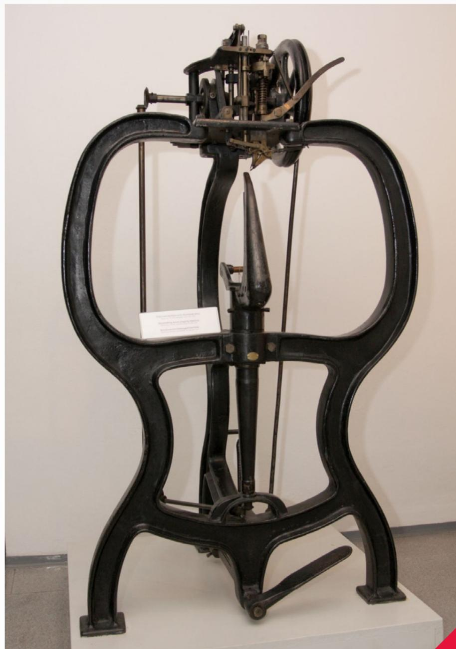
Shoemaking sewing machine of the Mc Key type from 1900, a prototype based on the patent by Lyman Reed Blake.
