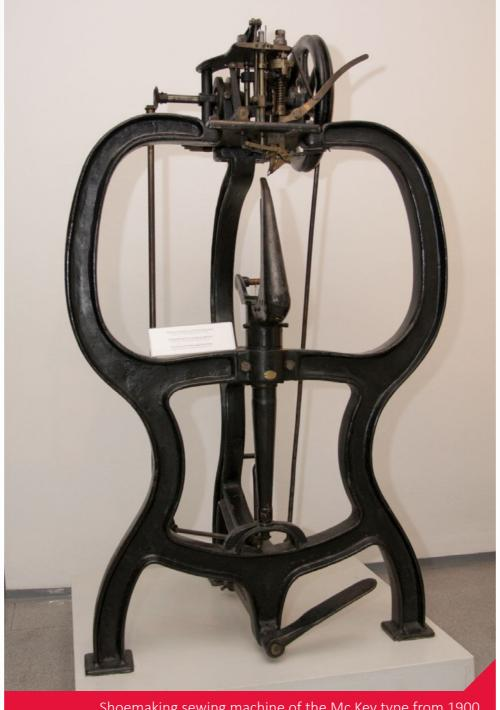
Shoemaking sewing machine of the Mc Key type from 1900, a prototype based on the patent by Lyman Reed Blake. Collection of the Museum of South East Moravia in Zlín.
